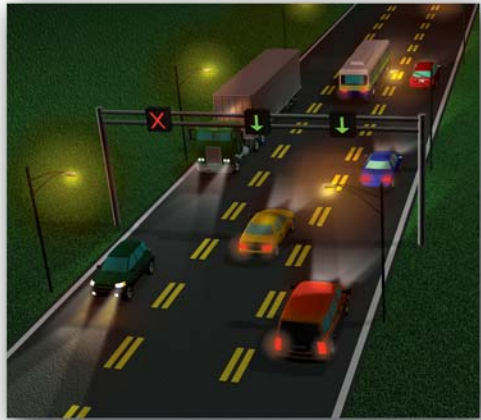
Lane Control Signal Lights
