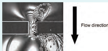
Figure 4. Early experimental observations and numerical predictions of 'stress fangs' within molten polyethylene; images taken from MPR experiments. (adapted from Lee, Mackley et al. , J. Rheol. , 45(6), 1261, 2001).
