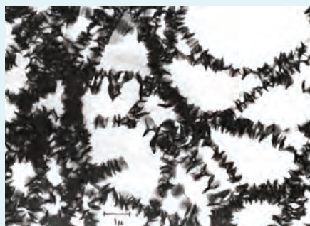
Figure 1. Transmission electron micrograph of 'shish-kebab' crystal structure of polyethylene, produced by an elongational flow-field (Mackley and Keller, Pure Appl. Chem. , 39, 193, 1974)
