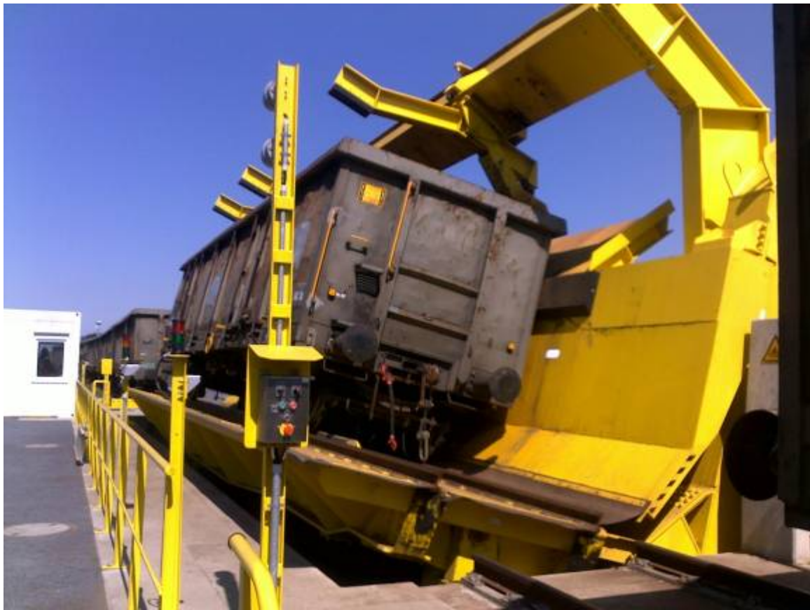
Picture 3: Wagon tippler, wagon started tilting
