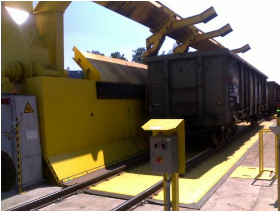
Picture 5: Wagon positioned in tipler, disconnected from locomotive and following wagon
