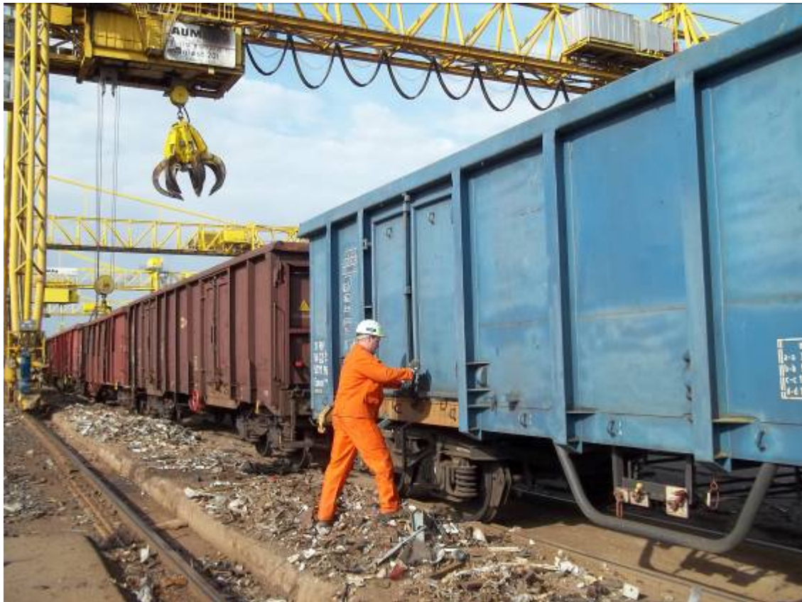
Picture 1: Opening the doors of scrap wagon, walk through dirt from wagon cleaning on the ground
