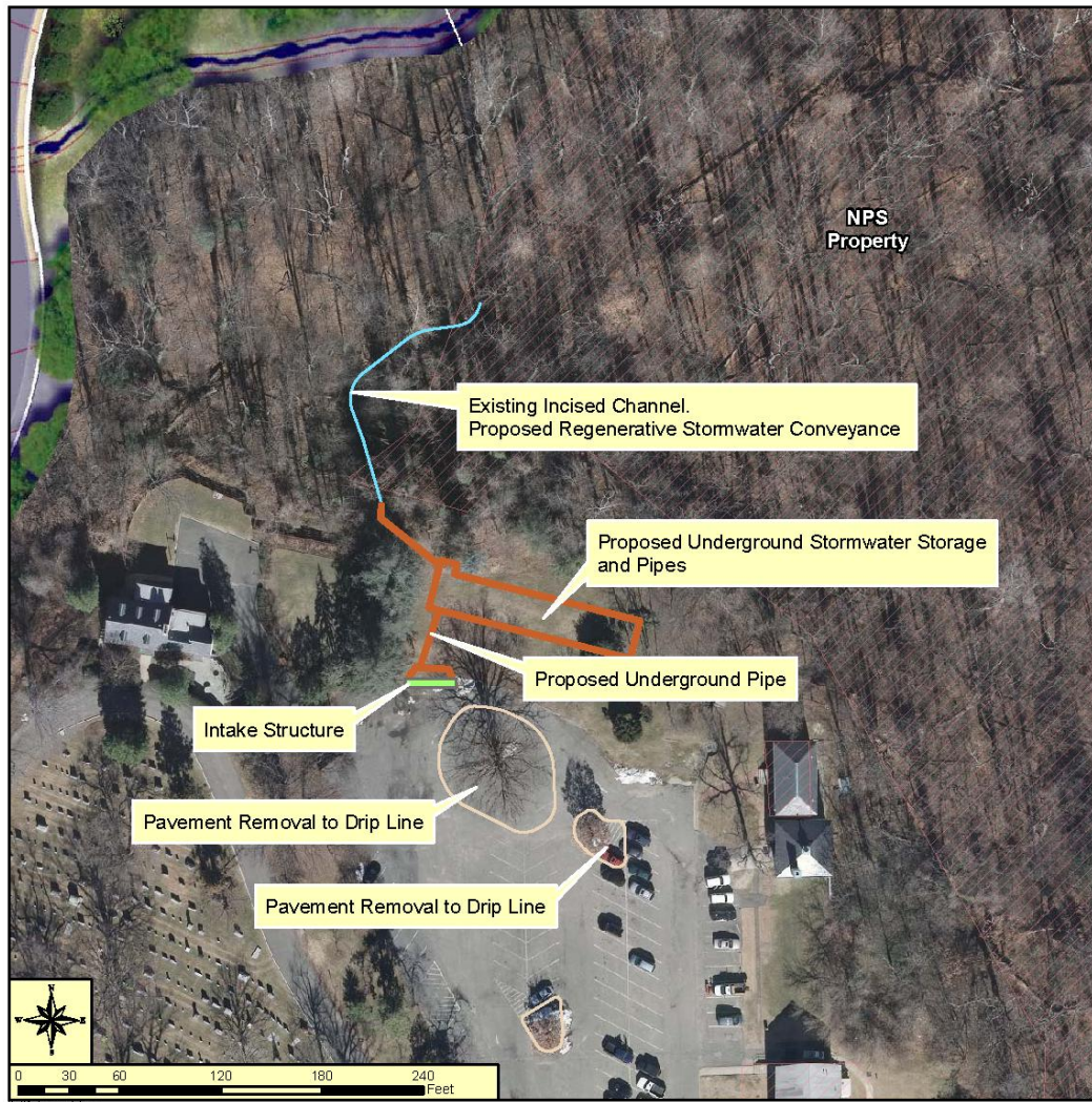
Figure 7 Main Features of Stormwater Management
