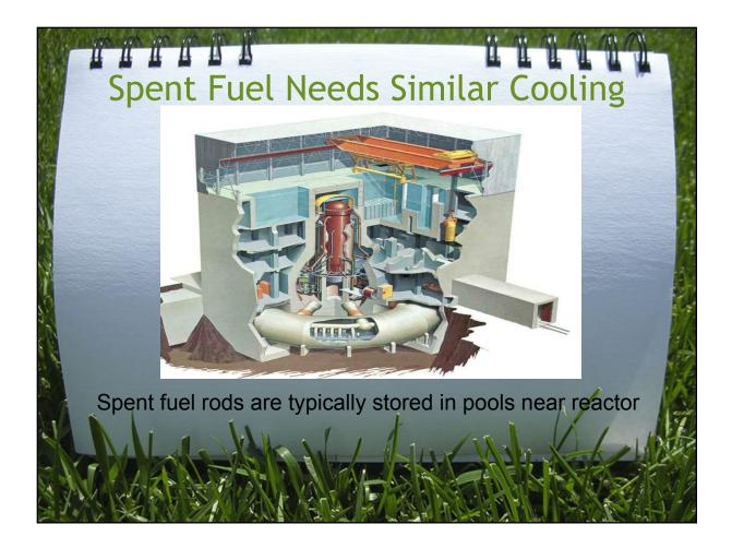
Spent fuel rod pool is in the far corner below the gantry crane in this illustration.
