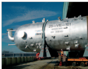
Chemical Reactors (MAN Diesel & Turbo)
