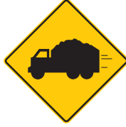
Truck crossing ahead
