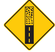
Pavement ends ahead
