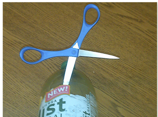
Figure 2: Note insertion point of scissors. Remember, scissors are sharp – be careful! First carefully insert scissors into the pop bottle at the point where the top taper ends.
