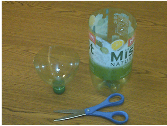
Figure 3: Remove the top of the bottle. Proceed to cut off the top of the bottle with the scissors. I have the label as a guide for a straight cut.
