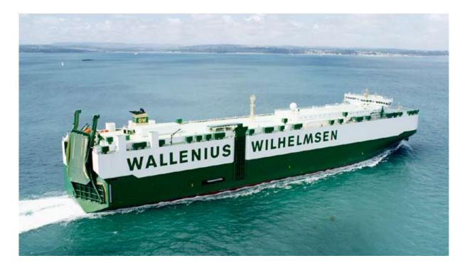
The LCTC (Large Car Truck Carrier) m/v FAUST has a capacity of 8,000 cars or a combination of 3,484 cars and 468 buses. With her 227.8 metres this capacity makes her one of the largest car carriers in the world. The vessel is built to the highest class of Lloyd's Regis-
