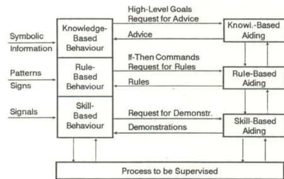
Fig. 2. Decision support systems classified according to the three-level model of Rasmussen (after Sheridan, 1987).
