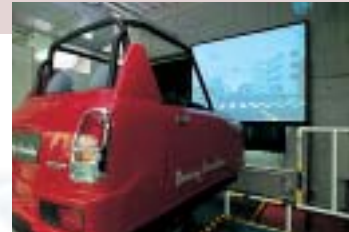
[ASV driving simulator] This simulator which makes us perform the dangerous experiments (to test safety) safely and precisely plays a vital role in Daihatsu's development process.
