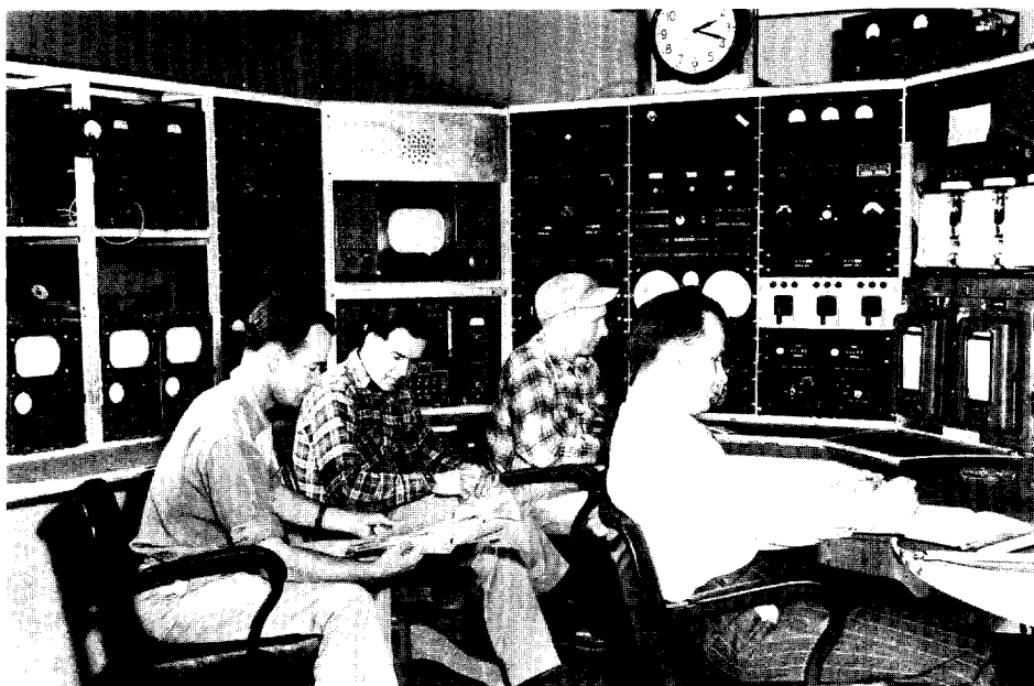
Fig. 2. (a) The original kiva, photographed from an Indian cave in the nearby wall of Pajarito Canyon, and (b) its control room, which was first housed in an existing shack. The racks contain controls for gradually separating and bringing together the parts of a critical assembly, displays of the long-counter responses that indicate neutron multiplication, radiation monitors that trigger a scram (automatic disassembly) if the level should become higher than intended, and a television screen for viewing the assembly. From left to right, Vernal Josephson, Roger Paine, Lester Woodward, and Hugh Karr. Paine and Woodward were military personnel who contributed invaluable to our critical experiments.
