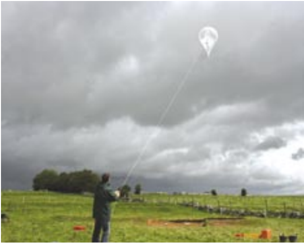
Figures 20 a-b: The use of balloons for low-level aerial photography a: Acquisition of aerial imagery using a Skyspot kite/balloon on an excavation trench at Carns, Co. Roscommon (Discovery Programme Medieval Rural Settlement Project)
