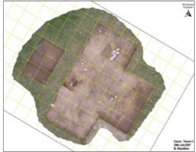
b: Ortho-rectified balloon-mounted imagery created using Topcon PI-3000 photogrammetry software (Discovery Programme Medieval Rural Settlement Project, 2007)
