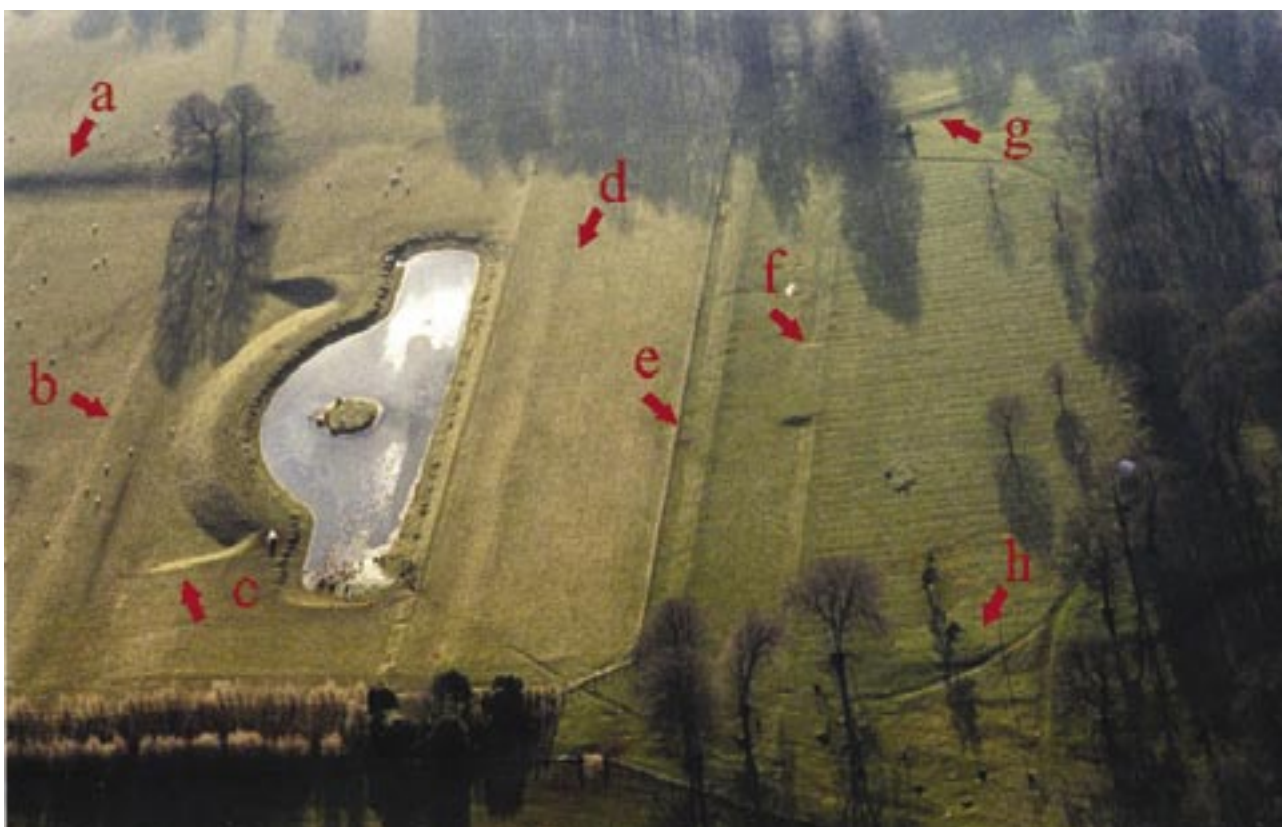
Figure 53: Aerial photography has considerable potential in locating designed landscape features as seen here at Russborough Park, Co. Wicklow. The pond and associated terracing (a, b, c, d, e and f) were mapped by Rocque in 1760 and were clearly visible in low spring light in 2001. (The survey by M. Gowen & Co. Ltd was carried out as part of a Conservation Plan commissioned by the Heritage Council)
