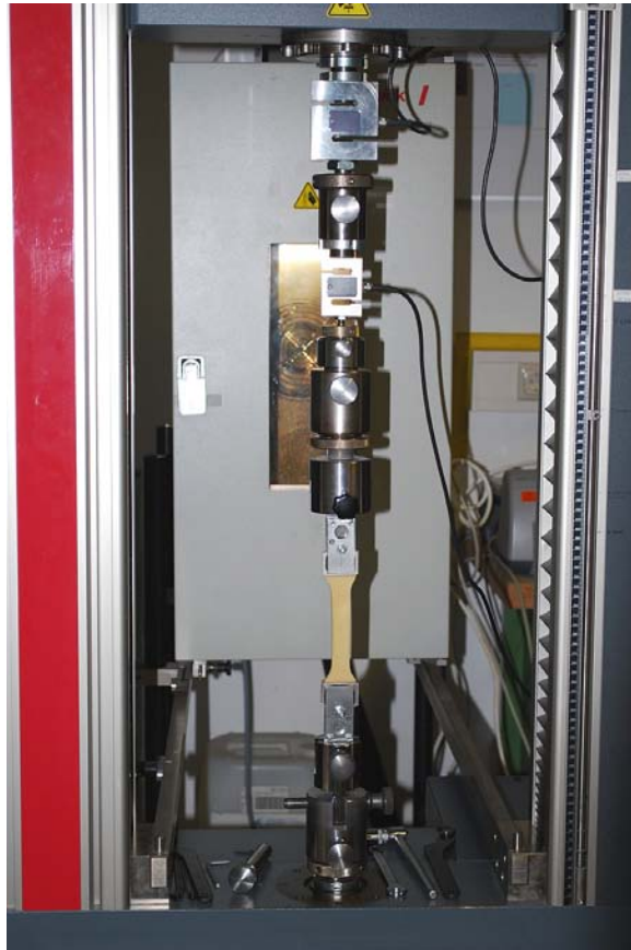
Figure 5. Wax sample during tensile tests.
