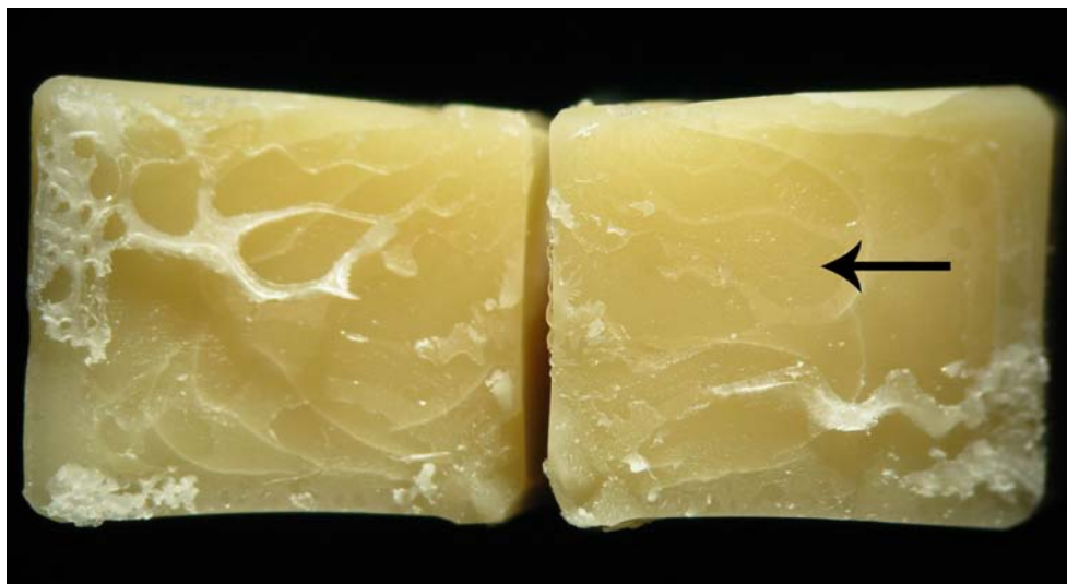
Figure 9. Fracture surface after bending test; arrow indicates glossy area where the wax surface has softened probably due to the influence of the solvent of the adhesive.
