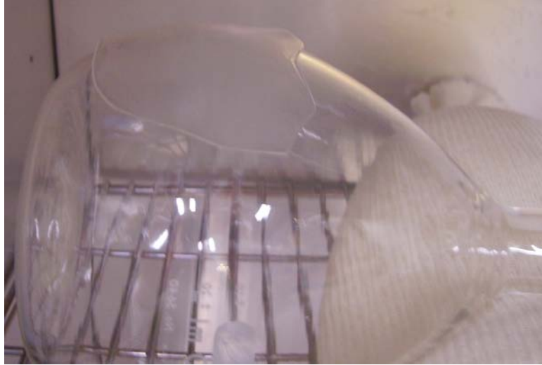
Figure 6: Shaping B-72 film on flask in oven
