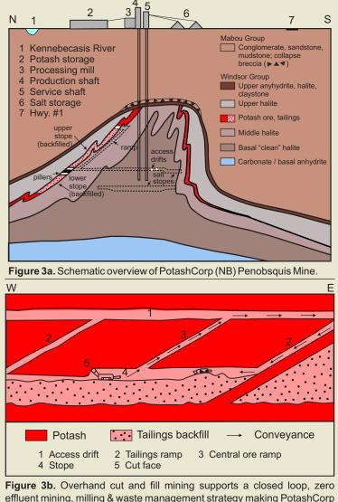
**Figure 3b.** Overhand cut and fill mining supports a closed loop, zero effluent mining, milling & waste management strategy making PotashCorp (NB) the only potash operation in the world that returns all its tailings and related waste materials underground.
