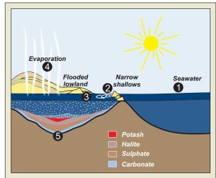
Formation of a typical potash deposit. Seawater (1) flows over narrow shallows (2) into a shallow basin (3), where it is evaporated (4). Carbonates, sulphates and the chloride salts of sodium (halite), potassium (sylvite) and magnesium (carnallite) precipitate out of solution onto the sea floor forming extensive evaporite layers (5).
