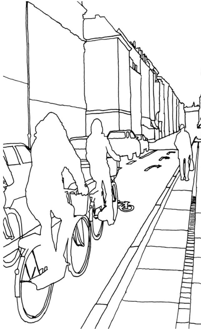
Above, bicyclists leave the cycle lane to merge with right-turning traffic at a junction. Along Store Kongensgade, the cycle lanes are 1.8 meters, but the turn lanes can be only 2.5 meters wide, which can be too narrow and cars sometimes do not leave enough room for bicycles to head straight across the intersection.
