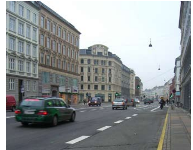
At Nørre Farimagsgade right after the junction with Ahlefeldtsgade, the cycle lane doesn't start until after the bus stop (marked in yellow). When a bus comes, the rules of the road are unclear - do cyclists wait for busses or go into traffic and then back to their lane?
