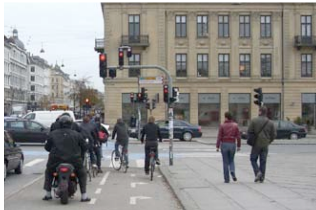
Along Dronning Louises Bro, a bicycle light and 1.5 meter lane is provided for both straight and right-turning cyclists.
