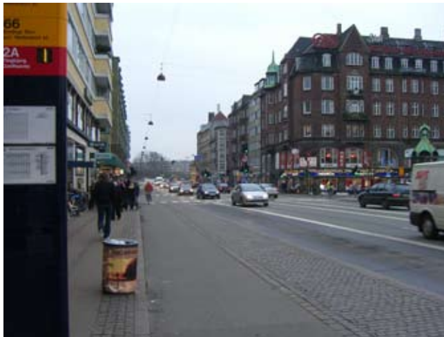
A 2 meter bus median and bicycle track on Torvegade opposite the Metro station that takes up the entire length of the block, allows quite a few people to wait if they wish. In practice, most people choose to wait on the sidewalk.
