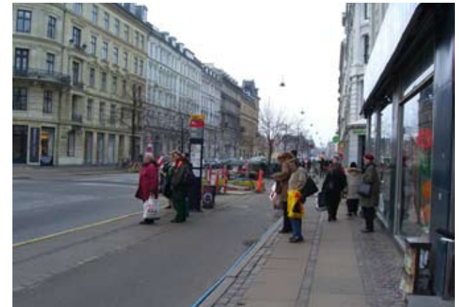
A bus island overflows with people waiting, blocking the sidewalk. At busy bus stops, a wider median may be warranted. Here it is 1.5 meters.
