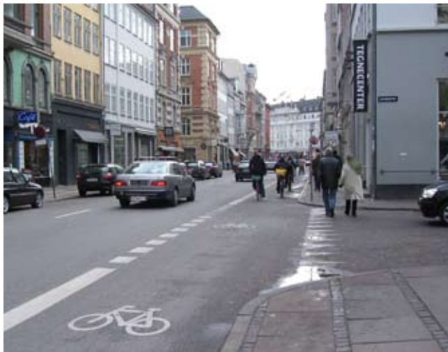
T-junctions along Store Kongensgade are usually marked with a dashed white line along the entire length of the junction with the side road, as in the photo above at the junction with Landgreven.
