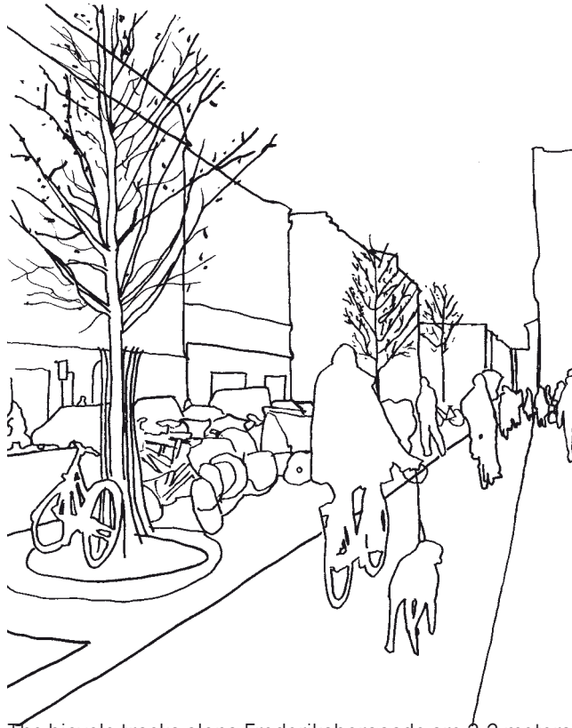
The bicycle tracks along Frederiksborggade are 2.2 meters, which feel quite comfortable to ride along even though they are heavily trafficked. This may have to do with the median, which is at the same height as the track itself, so it gives a passing cyclist more comfort and space to move around a slow cyclist. It is essential that cycle tracks have enough room so that people can pass each other easily. Above, a man takes his dog along for a bike ride, which is a typical scene in Copenhagen. Cycling in Copenhagen is just something that you do on a daily basis: to get groceries, to go to work, to visit a friend, or to “walk” your dog. It must be comfortable and convenient, or people will not do it. Streets with medians provide a good setting for bicycling and walking in Copenhagen, taking advantage of larger streets and using that space for people, not cars.
