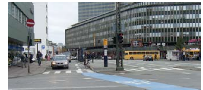
At Ved Vesterport and Bernstorffsgade, a blue marked crossing directs bicyclists across a confusing intersection.
