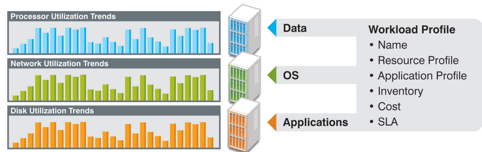
Figure 7. A workload profile captures invaluable information for planning and right-sizing the recovery environment.
