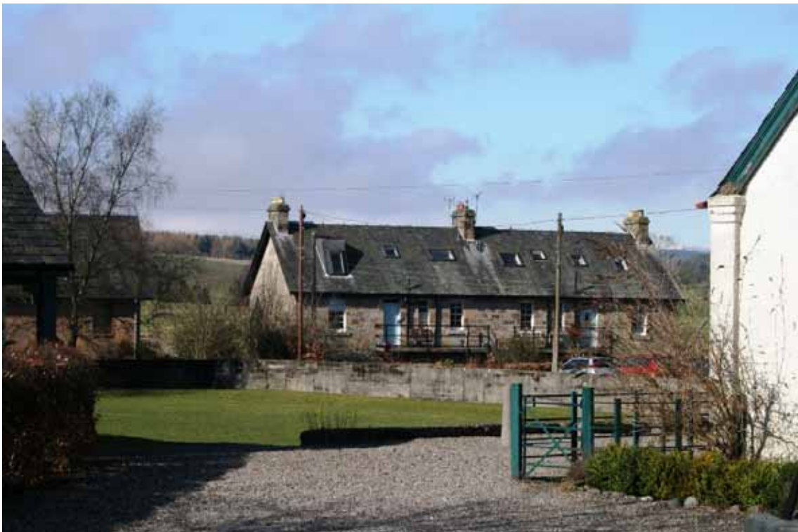
Fig 4: looking north-west across the former bowling green to the rear of Nos. 1-4 Allan View. This 2-storey block is reduced in scale due to the site levels dropping towards the river. The roofscape is prominent and important but has had inappropriate changes with rooflights in a variety of sizes and positions introduced, and a poorly designed dormer which interrupts the roofscape.
