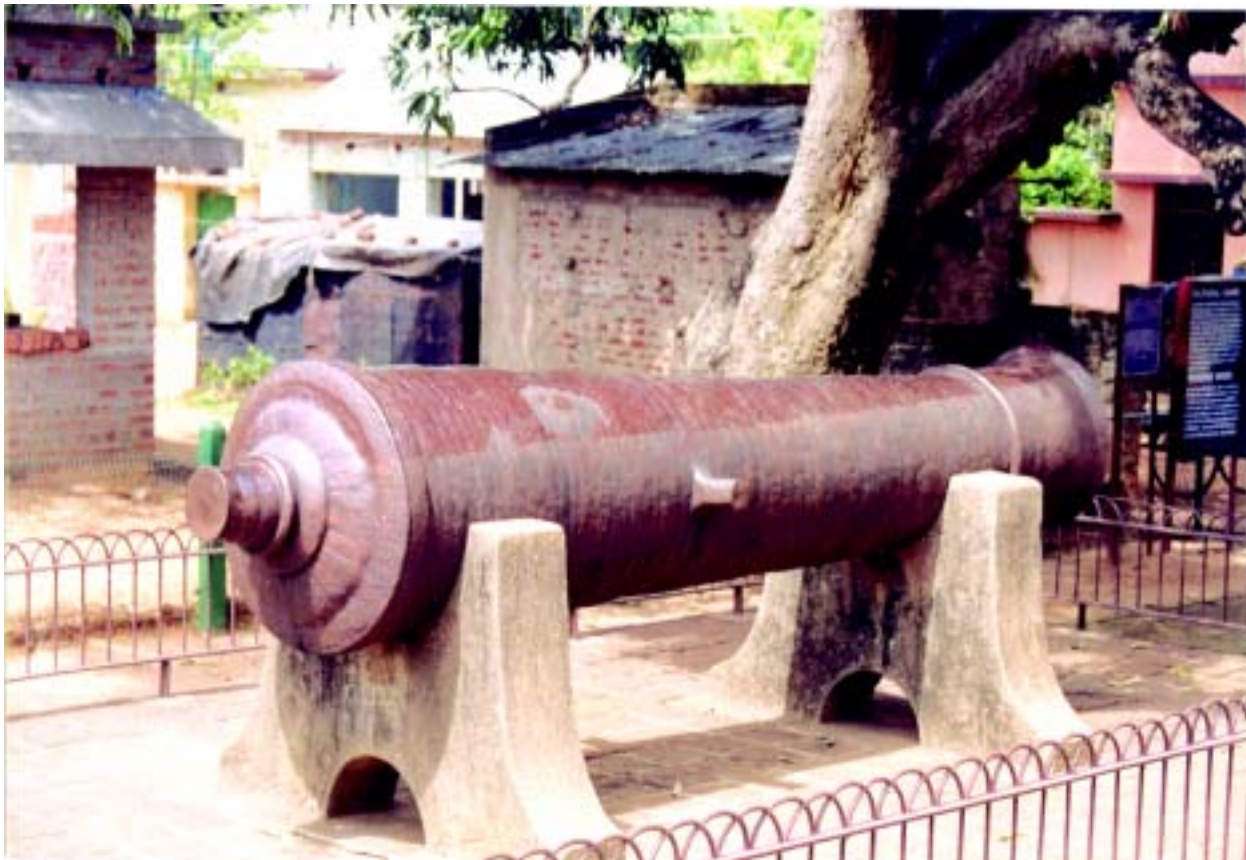
Fig.20: The forge welded iron cannon at Bishnupur, called Dalmardan
