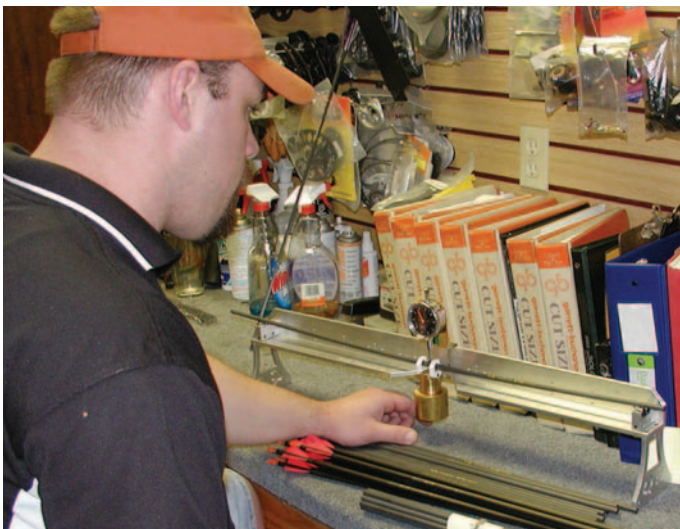
At Lancaster Archery, "Moose" Whitmoyer uses the spine tester by RAM Products to check the spine consistency of a dozen shafts. The device supports the shaft at two points 28 inches apart while a dial indicator measures the shaft deflection at its center caused by a 1.94 pound weight.
