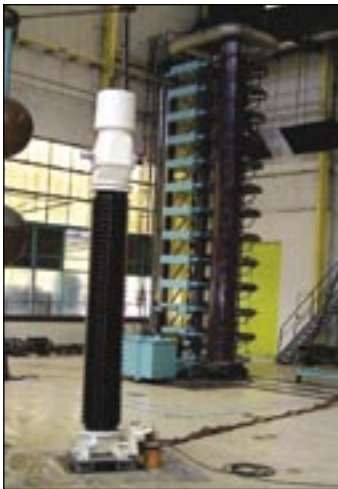
Fig. 3: Combined instrument transformer VAU-420 undergoing lighting impulse test of 1300 kV.
