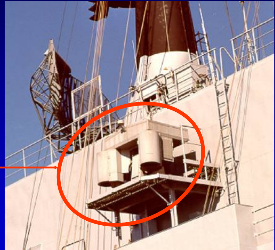
Nettuno System's ECM antennas, onboard the Italian-Navy carrier "Garibaldi"
