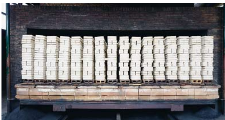
top left a. right Moulded bricks are made in wooden moulds, then dried and fired. The moulded bricks department was founded when the brickworks supplied new, ornamental terracotta brick for the renovation of the entrance to Tivoli Gardens in Copenhagen.
