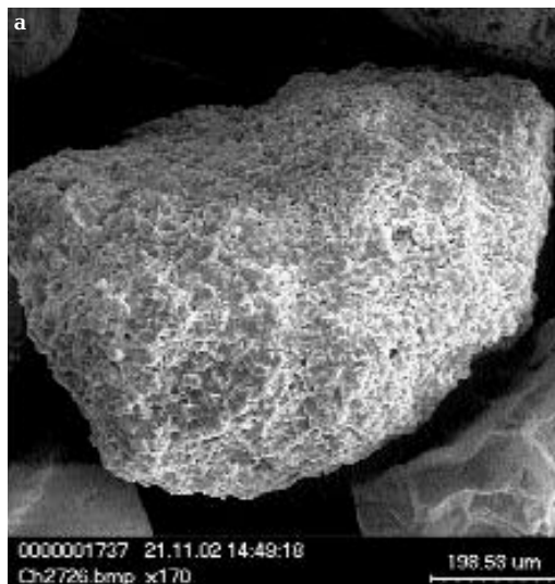
Fig. 5. BSE images of a 0.8 mm fragment of dolomitized limestone from clays of the Don moraine from southwest Moscow. (a) General view. (b) Detail of this fragment: segregations of twisted fibers of magnesian calcite around dolomite crystals.
