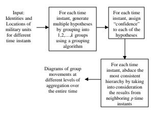
Figure 8. Algorithm for group identification and diagramming group motions.
