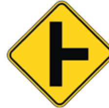
Side road enters highway ahead.
