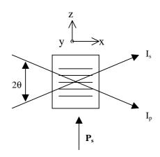
FIG. 4. Two beam coupling in  $KNbO_3$  crystals with the grating vector parallel to the z axis and beam polarizations in the x-z plane.
