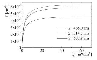
FIG. 6. The coupling gain  $\Gamma$  as a function of the light intensity  $I_0$  (modulation m = 0.06) for a fringe spacing  $\Lambda = 1.14 \,\mu\text{m}$  and tree different wavelength.
