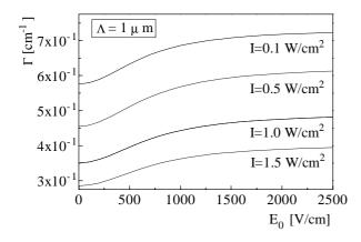
FIG. 7. The coupling gain  $\Gamma$  as a function of the applied electric field  $E_0$  for a grating spacing  $\Lambda=1 \ \mu m$  and four different light intensities  $I_0$ .
