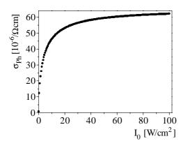
Fig. 2. Variation of the photoconductivity as a function of the illumination intensity  $I_0$ .
