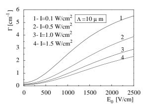
FIG. 8. The coupling gain  $\Gamma$  as a function of the applied electric field  $E_0$  for a grating spacing  $\Lambda$ =10 µm and four different light intensities  $I_0$ .
