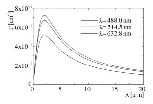
FIG. 5. The coupling gain  $\Gamma$  as a function of fringe spacing  $\Lambda$  for a light intensity  $I_0 = 70 \text{ mW/cm}^2$  and tree different wavelength.
