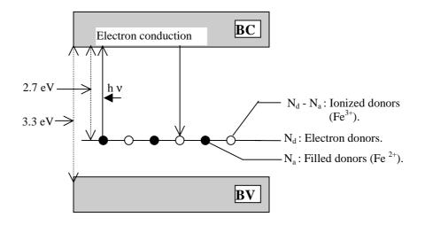
Fig. 1. Simplified band model of KNbO<sub>3</sub> for one electron donor center with density  $N_d$ . The donors are partially ionized in the dark and at low temperature (density  $N_a$ ).
