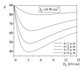
Fig. 9 Phase shift  $\phi$  between light and refractive index as a function of an applied electric field  $E_0$  for different fringe spacing  $\Lambda$ .
