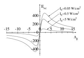
FIG. 3. Variation of space charge field as a function of fringe spacing for different light intensities  $I_0$ .
