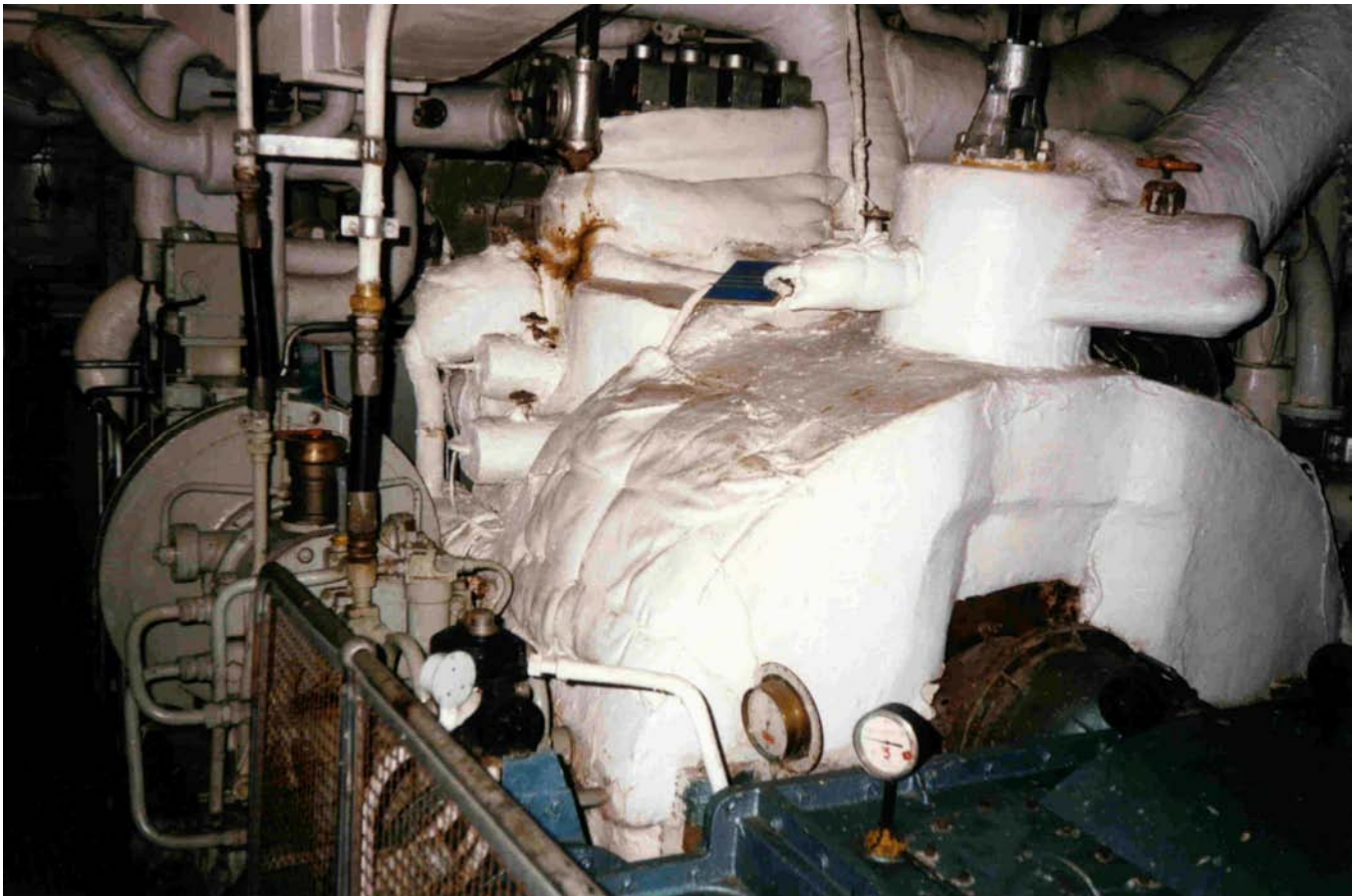
HMS Plymouth Port Main Turbine (Hull Stabiliser Hydraulic Pump in lieu of Cruising Turbine)
