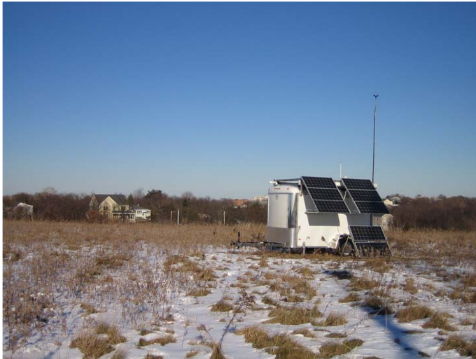
Figure 6 RERL SODAR Operating at Hull Landfill
