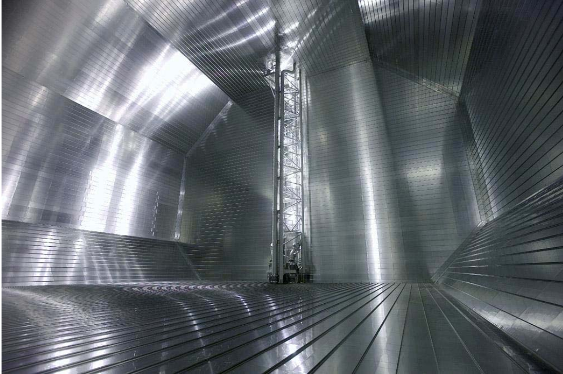
Figure 6-3 Membrane Tank – Courtesy GTT
