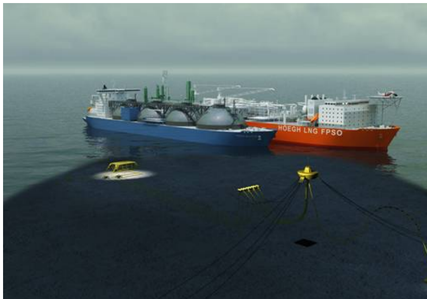
Figure 4-23: Side by side transfer – Courtesy Höegh LNG
