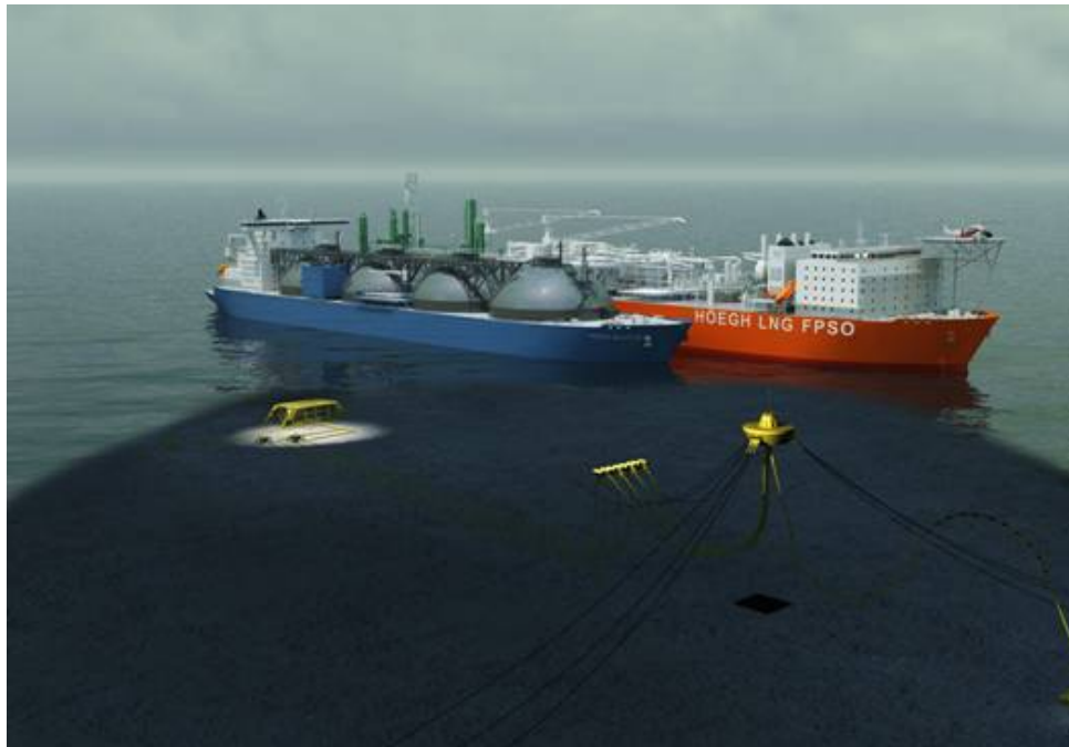
Figure 3-22: Side by side offloading (courtesy of Hoegh LNG)
