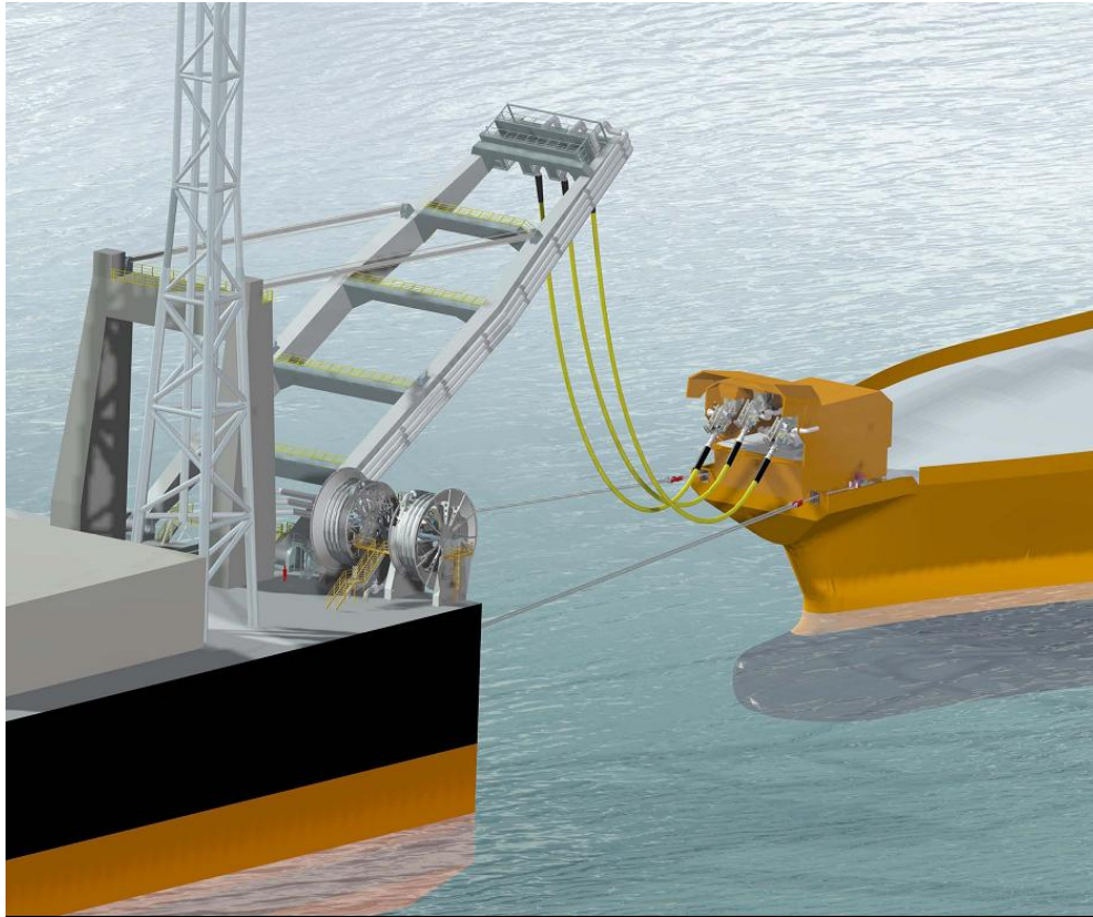
Figure 4-25: Aerial Hose Tandem Offloading System – Courtesy FRAMO
