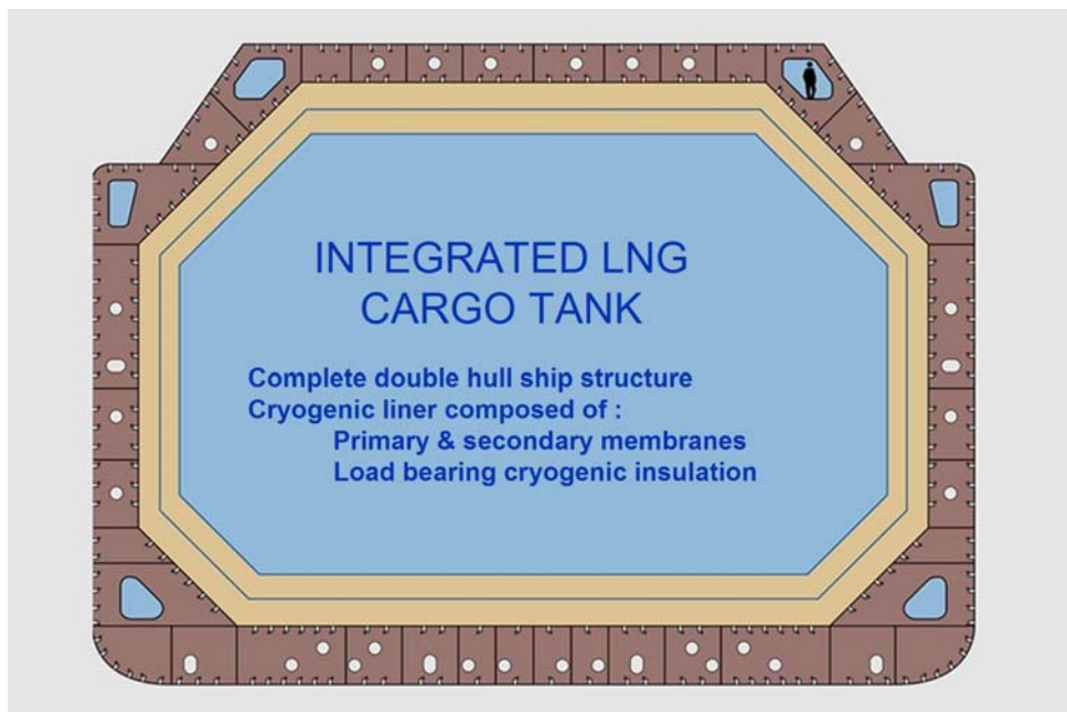
Figure 4-6: Generic Membrane Tank
