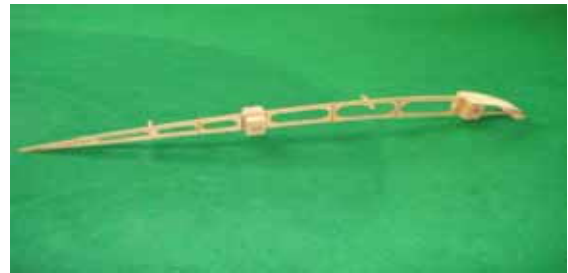
Holzrippen (Blériot, DH1, DH3, DH5, CV, C-35)
