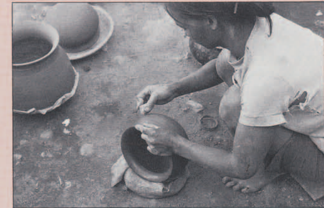
Figure 6e. The body of the vessel is burnished with a small rounded stone (idjidj) until the surface is smooth. The potter then incises lines of decoration around the vessel's neck with a bamboo stylus. The vessel then dries for a few days.
