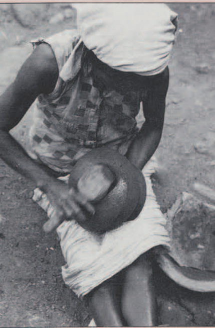
Figure 6d. When the vessel has dried to a leather-hard state, the potter removes it from its base. Pressing a stone anvil against the interior wall, the potter uses a wooden paddle (pikpik) to pat the base into a globular shape. A stripe of ocher (red mineral pigment, or pula) is painted around the perimeter of the vessel's upper body.
