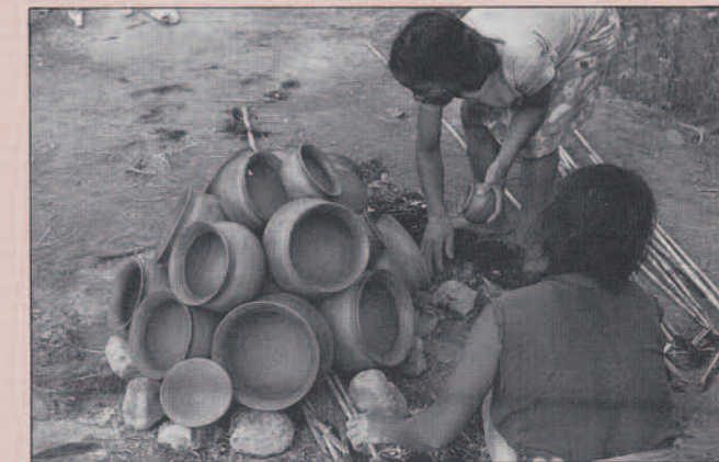
Figure 6f,g. Firing is done during the early morning or early evening hours, and takes place when several pots have been completed. Potters frequently pool their efforts and fire 10 to 20 pots together (6f). Large vessels are stacked at the base of the pile, while smaller pots are placed on top to ensure even heat distribution. Firing materials, including split bamboo, grasses, and rice stalks, are stacked in and over the pile (6g). The firing process lasts between 20 and 35 minutes, depending on the size and number of vessels.
