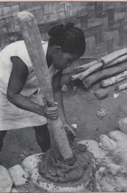
Figure 6a. Clay (soka) is collected from sources that are located in the walls of ricefields or in the midst of swidden plots, generally within 45 minutes' walk from the village. To prepare the clay, the potter removes large pebbles from the fabric and pounds the clay thoroughly. The clay is then shaped into a cylinder in preparation for the forming process.
