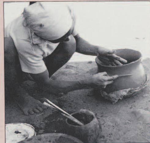
Figure 6c. The potter uses a bamboo wand (gilgil) to smooth the vessel walls and with a circular motion begins to form the vessel rim. A wet rag is used for the final rim-shaping process. After the vessel has attained its basic shape and the surfaces have been smoothed, the potter places the vessel in a shaded area to undergo its first drying phase. The length of the initial drying depends on the weather; it can last between six hours (during the dry season) and a few days (during the monsoons).
