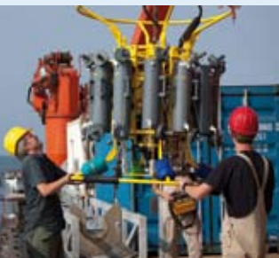
Scientists set up the water sampling device onboard a research vessel.
