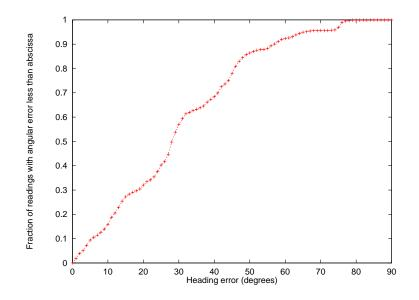
Figure 5.24: Accuracy of orientation measured using a single MPD
