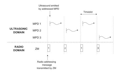
Figure 4.1: Operation of system using timeslots
