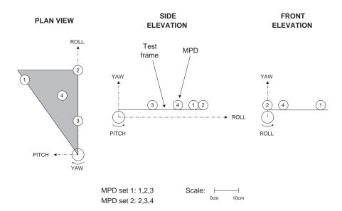
Figure 5.22: Test frame for orientation measurements
