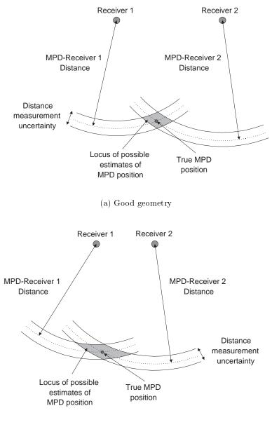
(b) Poor geometry
