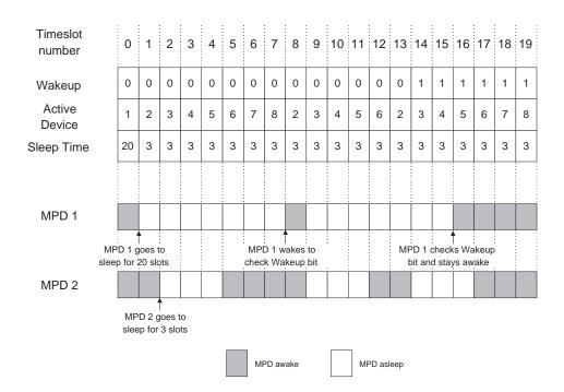
Figure 6.2: Behaviour of MPDs in sleep state
