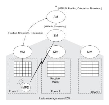
Figure 6.5: Tracker operation with several receiver matrices
