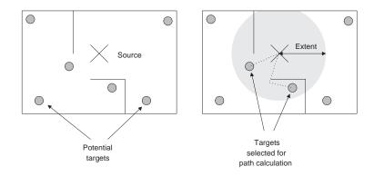
Figure 7.7: Simplifying bounded proximity queries using spatial indexing
