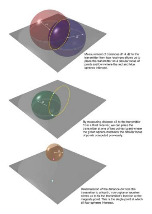
Figure 3.1: Multilateration in three dimensions
