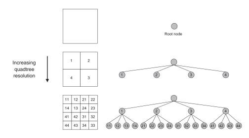
Figure 7.2: Quadtree data structure
