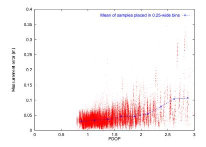
Figure 5.20: Variation of measurement error with PDOP
