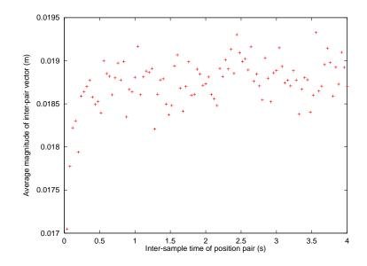
Figure 5.18: Temporal correlation between position measurements
