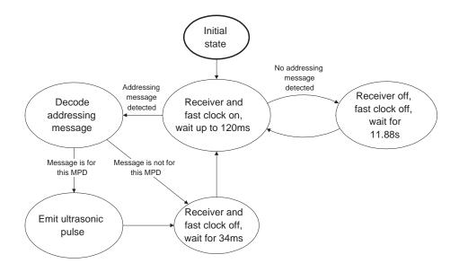
Figure 5.4: MPD operating state diagram
