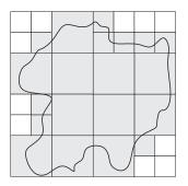
Figure 7.3: Maximal cover of a shape
