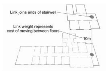
Figure 7.6: Modelling a building as a set of 2D floors
