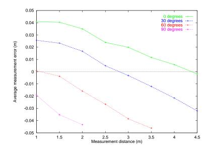
Figure 5.9: Accuracy of receiver distance measurements
