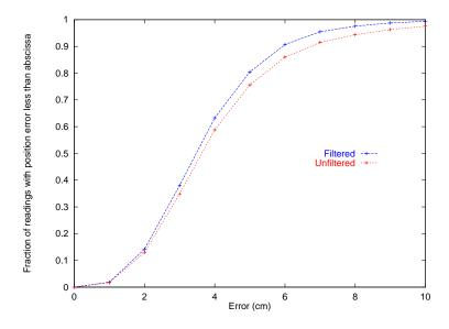
Figure 5.21: The effects of filtering using PDOP
