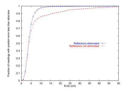
Figure 5.13: Accuracy of ultrasonic tracker
