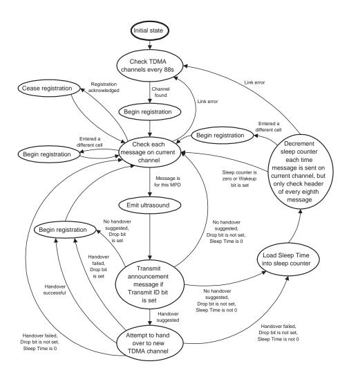
Figure 8.4: Simplified MPD operation
