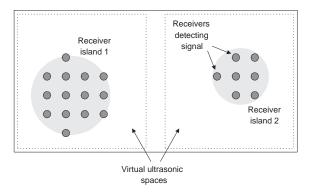
Figure 6.7: Identification of virtual ultrasonic spaces in a large room
