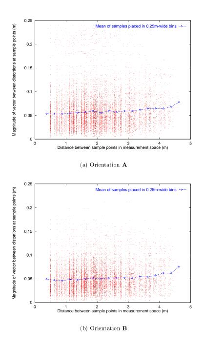
Figure 5.17: Spatial correlation of measurement space distortions
