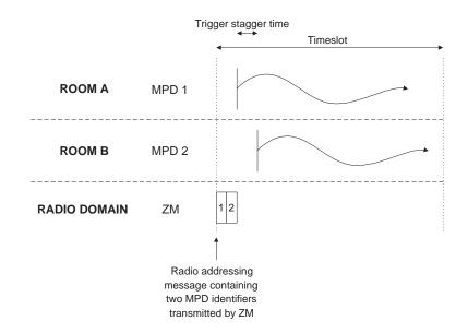
Figure 6.6: Staggered triggering of MPDs
