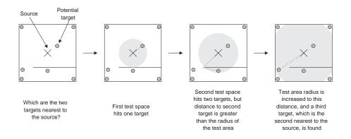
Figure 7.9: Simplifying unbounded proximity queries using spatial indexing
