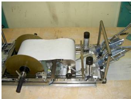
Figure 11. Light equipment for membrane containment erection
