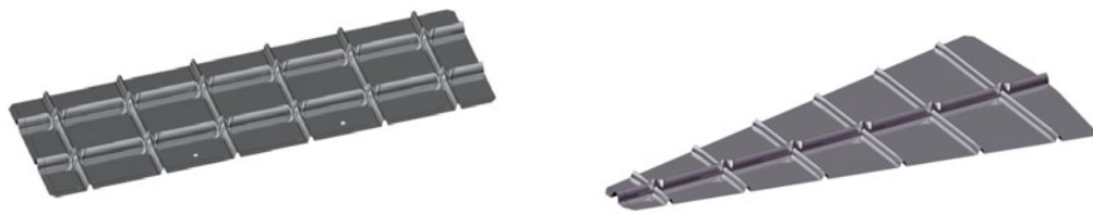
Figure 4. Primary membrane main elements
