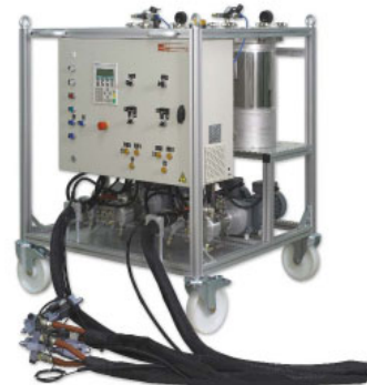
Figure 11. Light equipment for membrane containment erection
