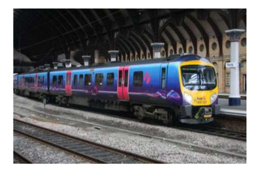
The Class 185 multiple units are a diesel version of Siemens' extensive and high-performing Desiro product range, having been built in Krefeld in Germany. They were purchased to provide the comfort and power required to operate inter-city routes across the Pennines and from Northern England to Scotland. The fleet is fitted with passenger and cab air-conditioning systems and provides a mixture of First and Standard Class accommodation.
