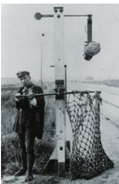
Loading and unloading of mail bags by a loading machine (1907) [from Postal Museum collection]
