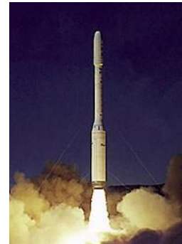
CASTOR and Orion Motors Boost Taurus
