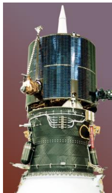
Lunar Prospector (STAR 37 Integrated Stage)
