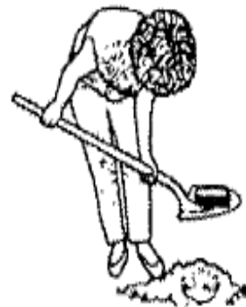
Figure 1b. Use a hand trowel, shovel or other garden tool. Trim out soil of uniform thickness to the recommended depth.
