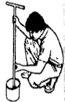
Figure 2. Place 10 to 15 soil cores into a plastic bucket; mix, dry, and transfer to a bag.
