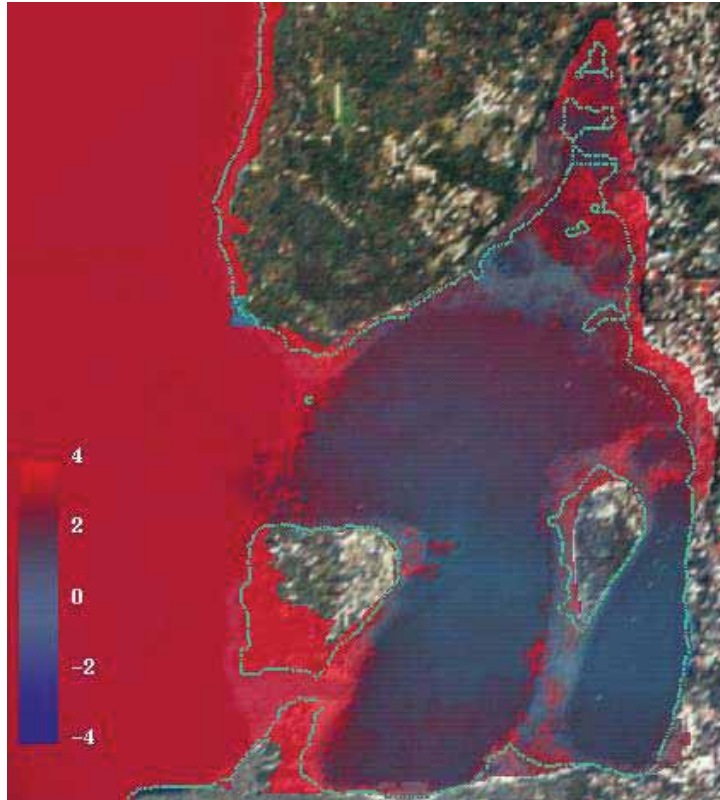
Figure 5. Maximum computed wave heights and inundation in the Port Vila Harbor for worst-case source scenario. The initial shoreline is shown as a blue contour line.
