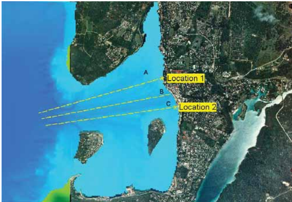
Figure 27: Sections A, B and C. Blue shading is of significant wave heights for TC Beni – the breaking zone over the steep bathymetric gradient outside the harbour is clearly evident
