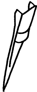
Blended Wing-Body; Bottom-mounted Propulsion
