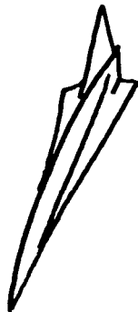
Government Baseline Vehicle Wing-Body; Bottom-mounted Propulsion
