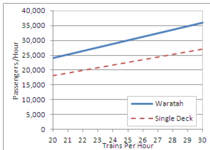
Figure 3.3: Nominal Train Line Passenger Capacity
