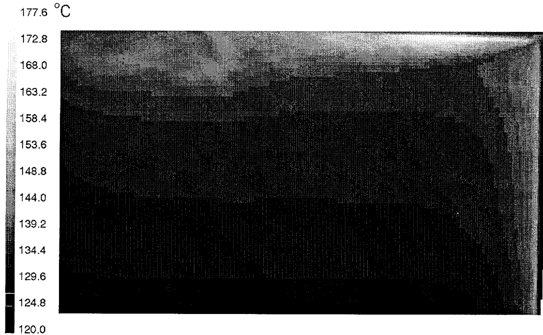
Figure 14. Temperature Contours Below the Fuel Racks ( z = 0.1\text{m} )
