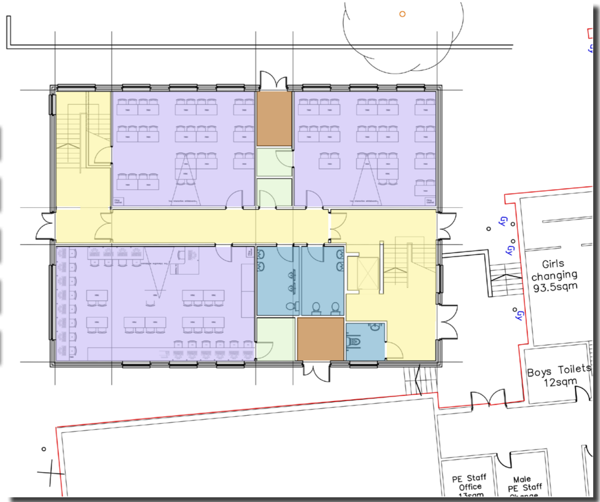
Ground floor plan showing the general arrangement of the spaces within the Classroom Extension
