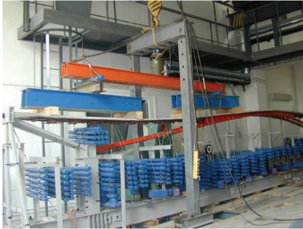
Figure 5: Static model – ultimate load
