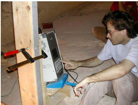
Figure 4. The Minolta 900 on a specially built rig allowing the scanner to remain perpendicular to the scanned surface (i.e., parallel with the surface normal of the resulting model).
