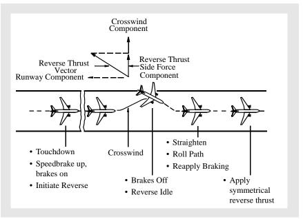
This figure shows a directional control problem during a landing rollout on a slippery runway with a crosswind. As the airplane starts to weathervane into the wind, the reverse thrust side force component adds to the crosswind component and drifts the airplane to the downwind side of the runway. Main gear tire cornering forces available to counteract this drift are at a minimum when the antiskid system is operating at maximum braking effectiveness for the existing conditions.
