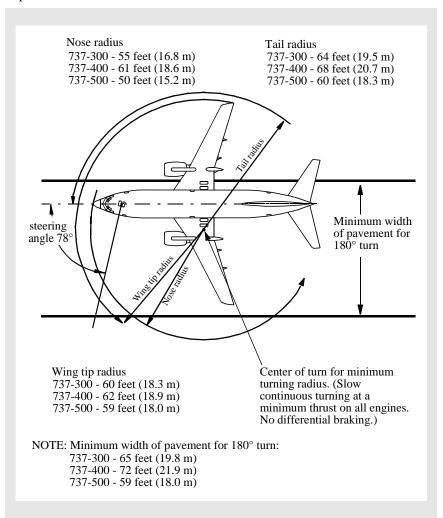
CAUTION: Do not attempt to make a turn away from an obstacle within (15 feet/4.6m) of the wing tip or within (25 feet/7.6m) of the nose for the 737-300/500, or (22 feet/6.7m) of the nose for the 737-400.
