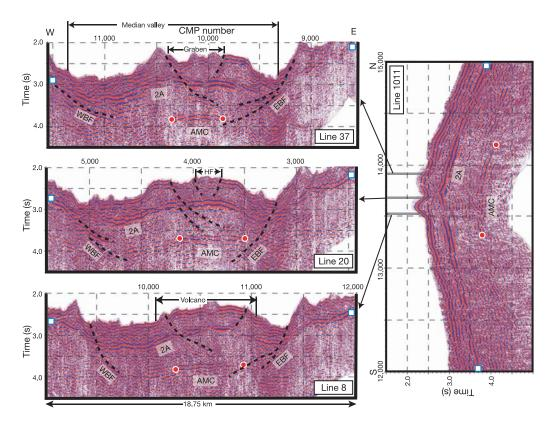
**Figure 2** | **Seismic reflection images of the AMC and faults.** Seismic sections across the ridge axis (lines 8, 20 and 37) and along the ridge axis (line 1011). The vertical exaggeration is 1:1, assuming a velocity of 5 km s<sup>-1</sup>. Blue and red ripples represent positive and negative trace amplitudes, respectively. Red circles show the limits of the AMC reflector, blue squares mark the layer 2A reflector and dashed black lines indicate principal faults
