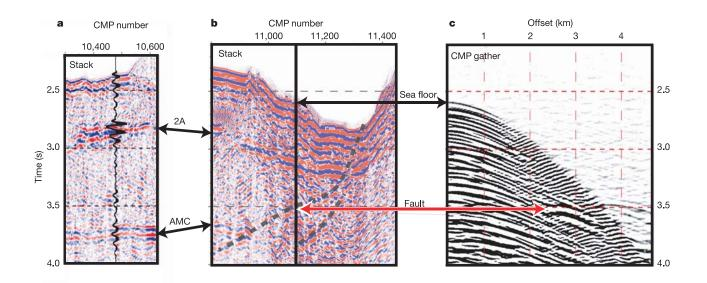
**Figure 3** | **Fault and AMC reflector details.** Detailed seismic sections from line 8. **a**, Section showing the sea floor, layer 2A and the AMC reflector. The AMC reflector has the opposite polarity of the other reflectors. The black wiggle trace highlights the polarity of different events. **b**, The EBF, enlarged
