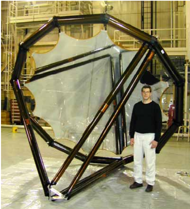
Active inflatable-rigidizeable spacecraft structures (NASA, JPL, DoD, L'GARDE, ILC Dover)
